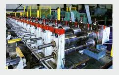
Inventory / Rollformers / #3246 24 Stand x 1-1/2" RLM Duplex Type Panel Rollformer
